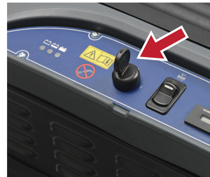
9. Release the traction lever, lift the side broom by and turn off the machine with the ignition key "0".
