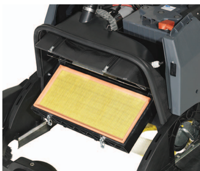
12. Remove and clean the dust filter as indicated into the manual.
