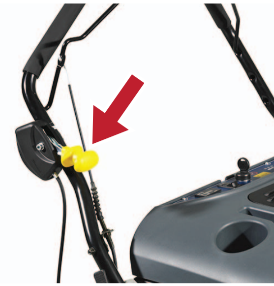
4. Lower the side broom by pulling the lever backwards.
