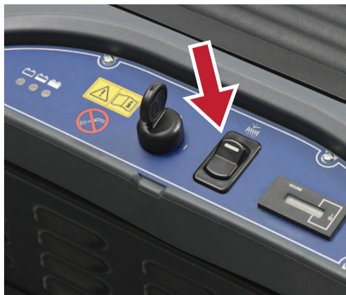
7. Activate the filter shaker switch every 10 min.
