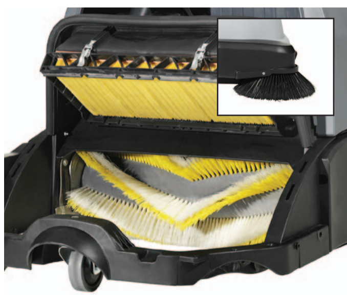
11. Check the main and side broom and remove any debris like straps, rope etc..
