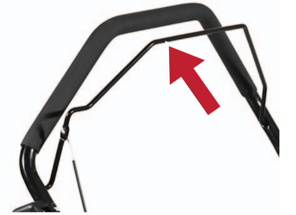
5. Activate the traction by pulling the lever.
