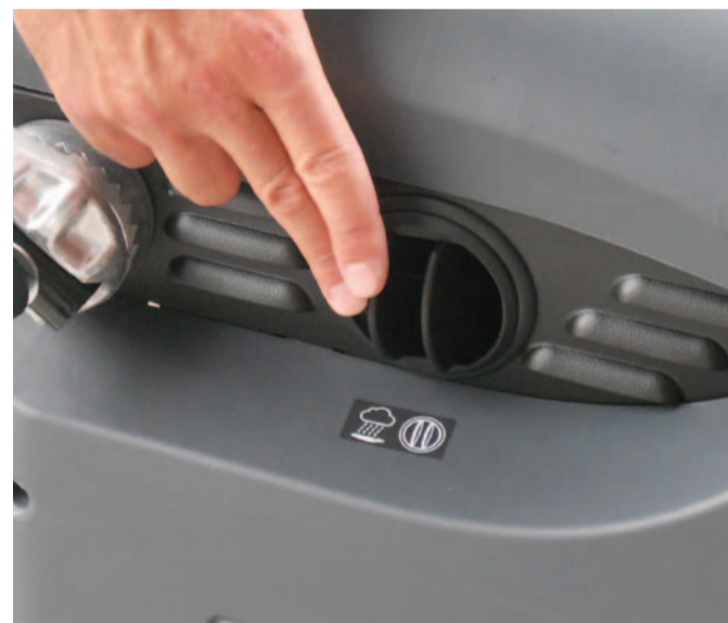
8. When operating on wet floors, open the "wet by-pass" port to avoid damaging the dust filter. Close the "wet by-pass" port to restore proper vacuuming.
