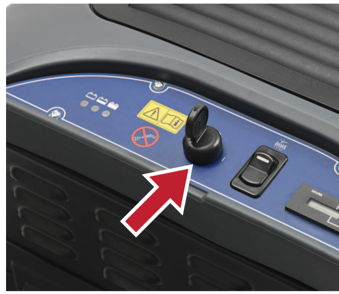
3. Turn the ignition key to "I" without pulling the drive control lever.
