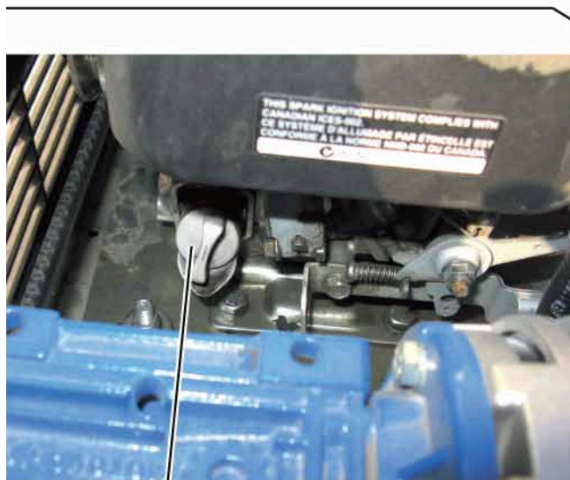
Engine oil level inner check plug
